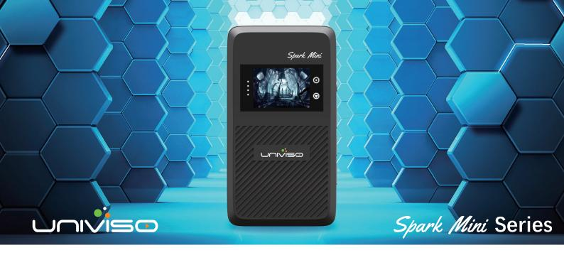
**Spark Mini** series live broadcast terminal is a high-performance live broadcast terminal specially designed for modern lightweight live broadcast needs in the Univiso live broadcast product family. It integrates broadcast-grade HEVC/AVC video compression algorithm and intelligent multi-link aggregation technology, and realizes low power consumption and low latency miniaturization design while ensuring high-definition audio and video transmission.
